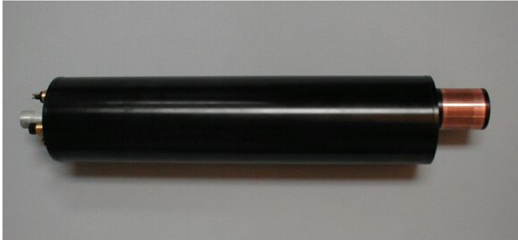
Figure F-10: The ISUS with Biofouling Guard
