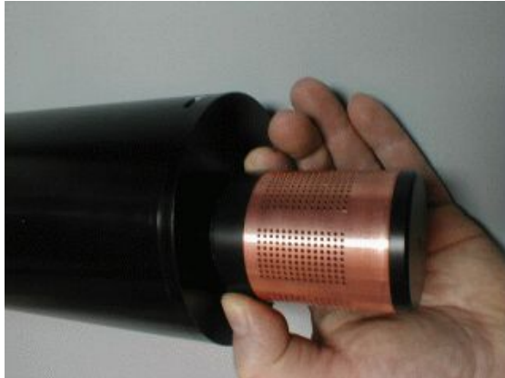
Figure F-9: Mounting the guard
