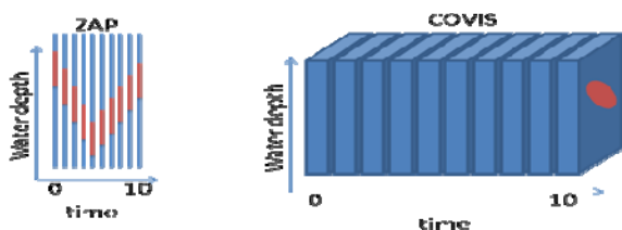
Figure 6-1. Contrasting data rates and dimensions of VENUS's ZAP and our proposed COVIS for 10 time increments shows the greater data rates of COVIS and that it produces 3D volumes instead of 1D lines. The data point of interest is mostly hidden in this view of the volumes.
