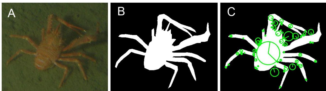
Figure 3. Example of the SIFT processing for the identification of a squat lobster ( Munida quadrispina ) within a digital still image at VENUS cabled observatory. Sequences of digital image products obtained by the automated processing are: (A) The original RGB image; (B) Binarized mask of the extracted animal; and finally, (C) SIFT features extracted in green ( i.e. , those considered as belonging to the object had the centre of the features located within the white mask area of B).
