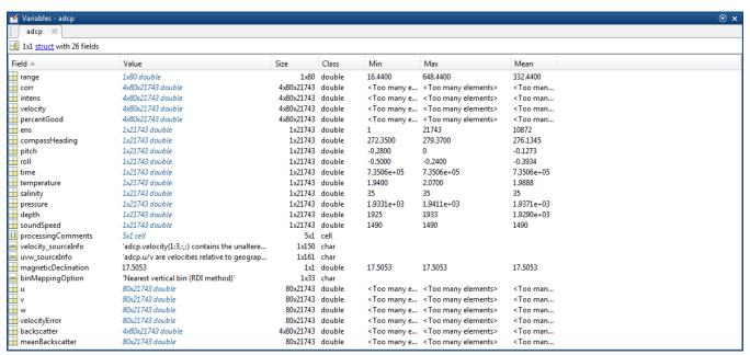
range: vector of distance to each bin centre. If bin mapping compensation for tilt is active, then the bins are moved so that ADCP.range is now the
